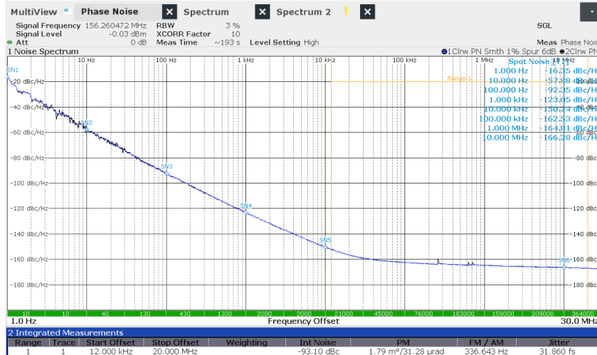
Figure 1. LVDS output phase noise plot @156.25M
